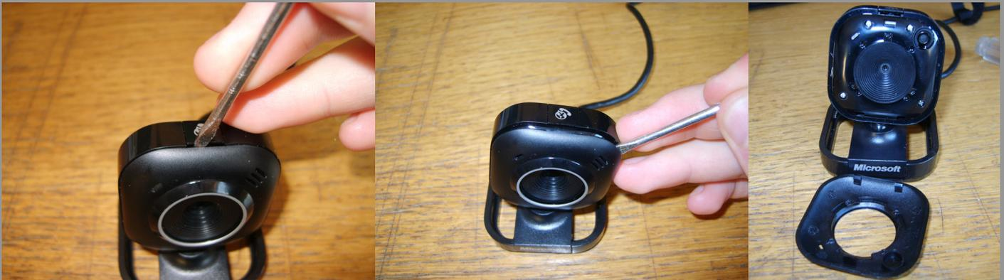
1. Take your 2000 and remove front fascia by placing a knife or thin screwdriver in the gap next to the button on the top. Apply a little pressure to pull the front fascia off, and work your screwdriver round the fascia.
