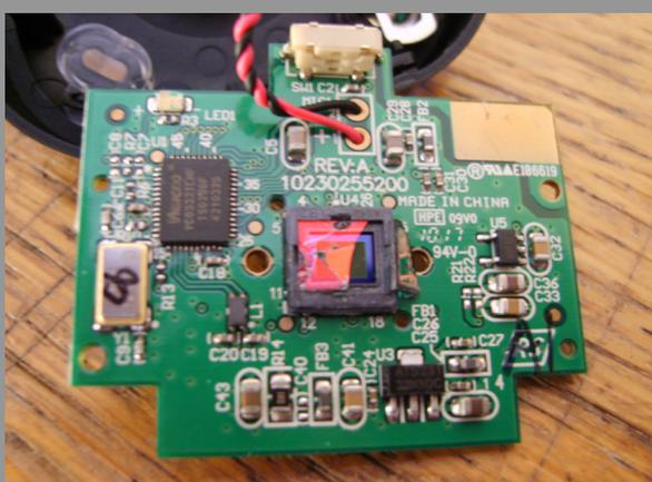
9. The CCD chip is revealed and that red tinted glass cover you see is the IR filter. There are four inlets in the plastic surround; you can insert a very thin knife or jewellers file into these, and careful work the glass plate off. I unfortunately cracked mine and the glass splinters scared the CCD chip ruining the camera. Be very careful!
