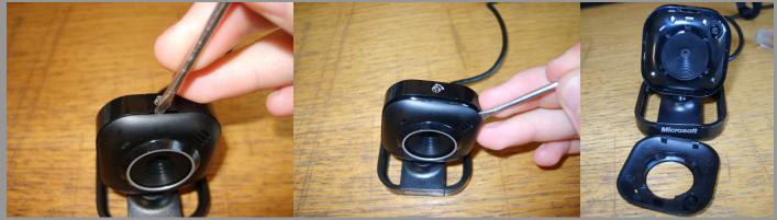
1. Take your 2000 and remove front facia by placing a knife or thin screwdriver in the gap next to the button on the top. Apply a little pressure to pull the front facia off, and work your screwdriver round the facia.
